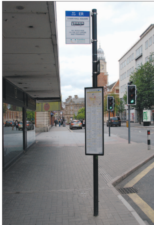
Above: Where no shelters exist, two pole-mounted cases were fitted and the Where to Board adapted to suit. The linear diagram and timetable went in the other case. This stop is alighting only but still has a Where to Board to help passengers on the next phase of their journey.
